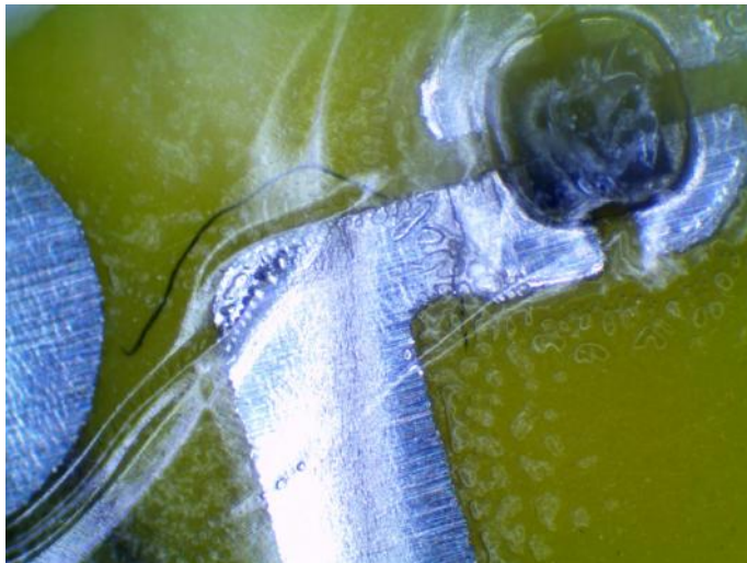
Figure 10: Web Inlay Transponder at Higher Magnification (Photo: Smartrac).
