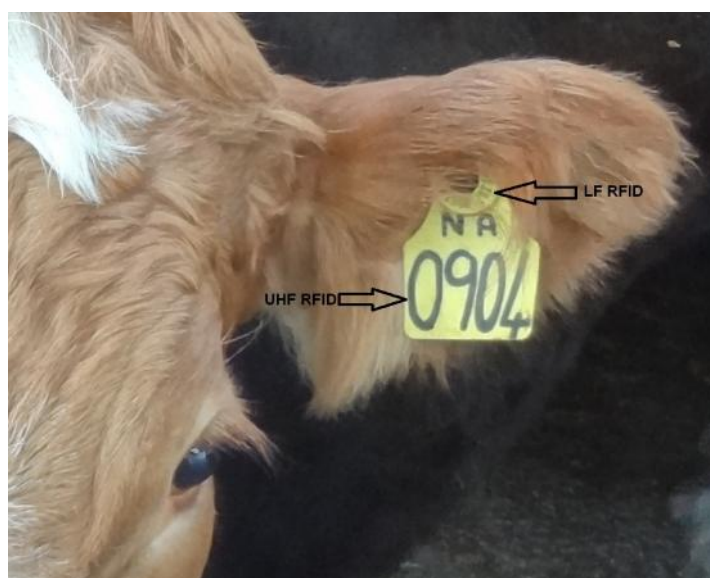
Figure 15: Dual Tag produced by ScotEID for experimental purposes.
