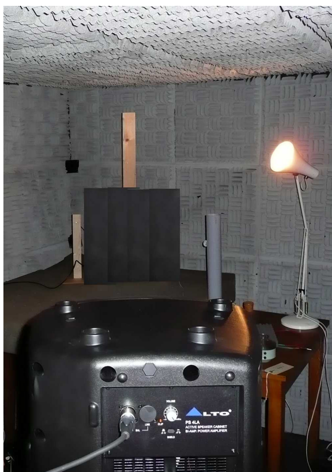
Figure 25: Immunity test system (test object masked out)
