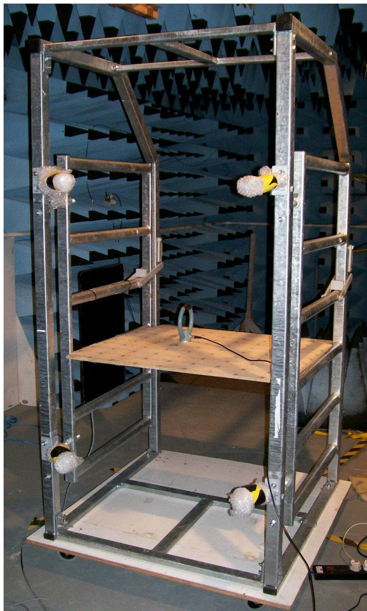
Figure 1.2-1 Tubular fencing kiosk used for the purpose of this study
