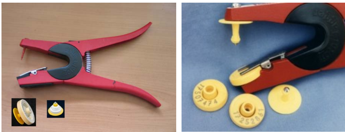
Figure 13: Example of pliers for the application of electronic ear-tags
