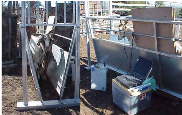
Figure 11: Dynamic reading of goats with the antenna placed on the left side of the race way
