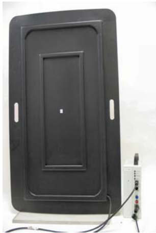
Figure 10: Stationary reader and transportable antenna
