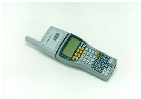
Figure 5: Example of a two piece hand-held programmable reader
